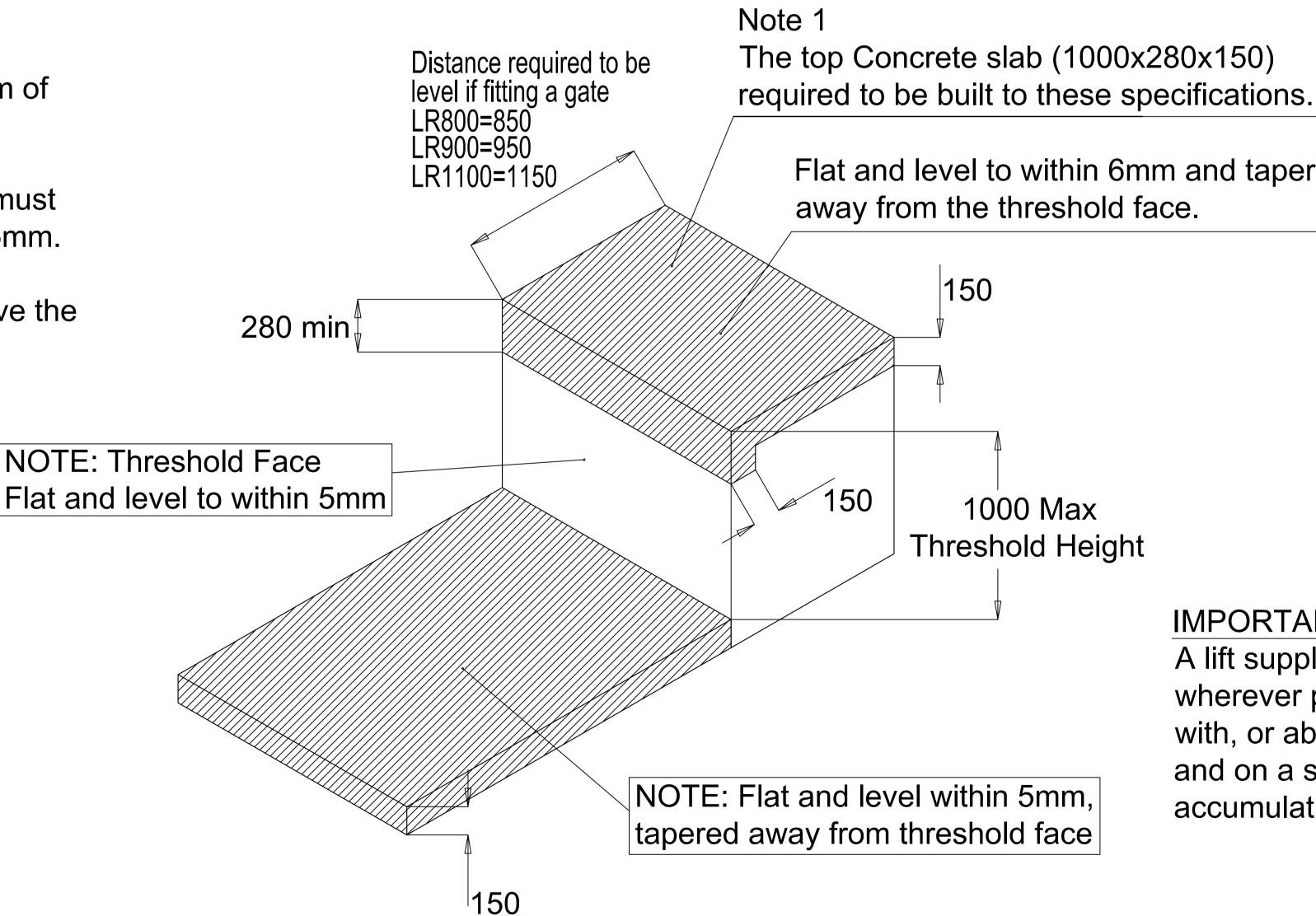
Flat and level to within 6mm and tapered away from the threshold face.
